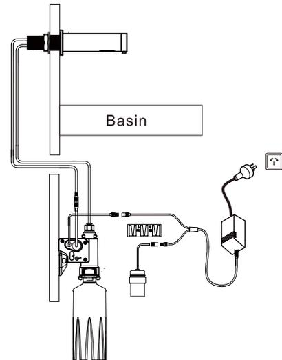
If AC/DC with battery back up, plug battery box into transformer and then plug in to mains socket.
