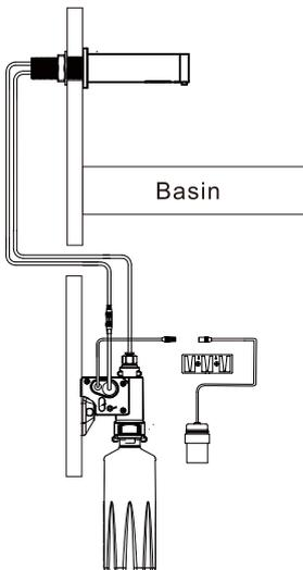
If battery only, plug battery box into power cable.
