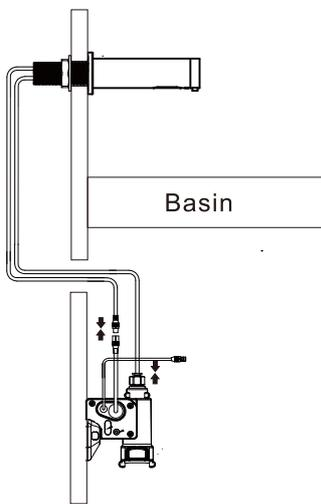
Plug the soap hose and control cable from the spout into the pump and controller.
