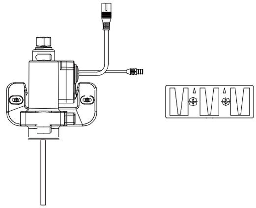
Screw the two brackets in suitable position under the basin making sure the hose and control cable can reach.
