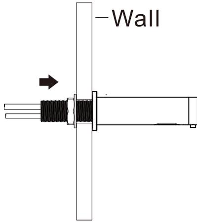
Place hose and control cable through the wall, then tighten nut to secure soap dispenser.
