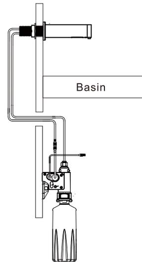
Fill with liquid soap and clip soap container into the pump and controller unit.
