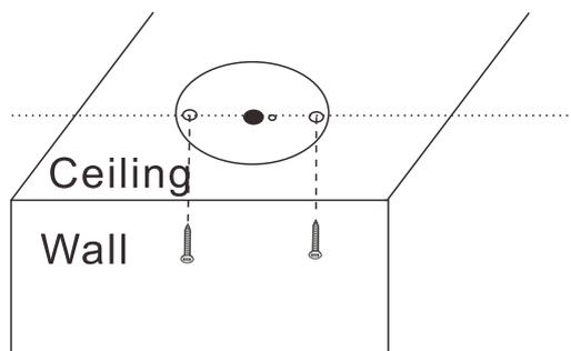
3. Twin or Trough urinals: refix the sensor plate using the 2 screws, **ensure sensor plate screws are aligned facing the wall.** (Before refixing make any changes if required to flush time or preflush settings, refer to page 4 and 5)
