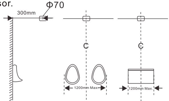
2. Remove the screws from the sensor plate and install the flush box into the ceiling using the screw clips. (Ensure the sensor screw holes are aligned as shown in 3)
