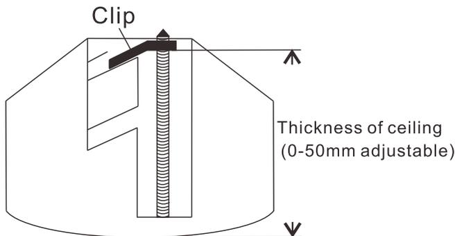
2. Remove the screws from the sensor plate and install the flush box into the ceiling using the screw clips. (Ensure the sensor screw holes are aligned as shown in 3)
