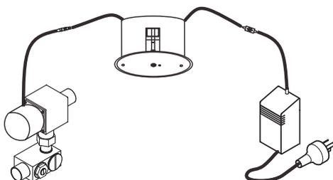
4. Connect solenoid valve to sensor (black plugs) and connect sensor to transformer (white plugs). Connect to power only when installation is complete, system will then run test and be ready to use.
